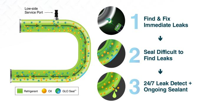
When the system is scanned with a **UV leak detection lamp** the leak will glow brightly. Scan the system periodically to find new leaks. Small, hard-to-find leaks hurt system performance and will eventually lead to total compressor burnout. Both dye and sealant can remain safely indefinitely, for **24/7 continual leak detection and ongoing sealing.**
